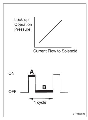
The current flow to the solenoid is controlled by the duty ratio\* of the ECM output signal. The higher the duty ratio becomes, the higher the lock-up hydraulic pressure becomes during the lock-up operation. \*: The duty ratio is the ratio of the continuity to non-continuity in one cycle.
